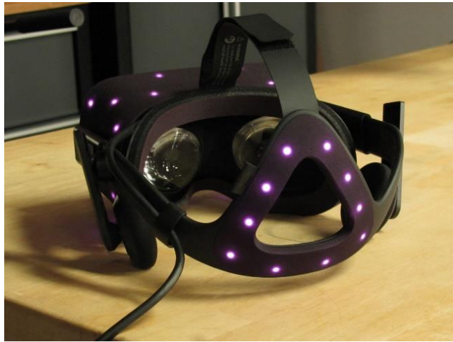
Figure 10 Oculus Rift Infrared Points (ifixit, 2016)
